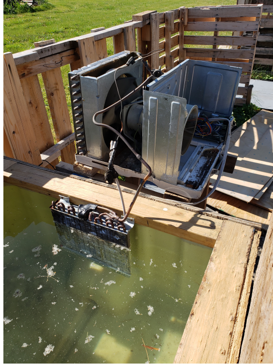
Figure 3: AC unit coil placement in the agricultural crate plunge
